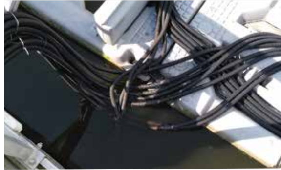
FIGURE 9.16 Biofouling on submerged connectors and cables
