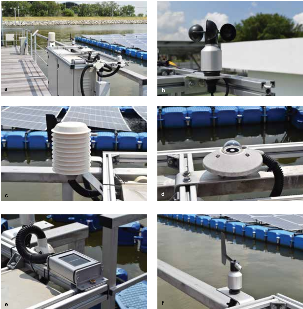
FIGURE 9.2 Meteorological station close to FPV system (a) and types of sensors: (b) wind speed sensor, (c) humidity sensor, (d) pyranometer, (e) Si-sensor, and (f) wind direction sensor
