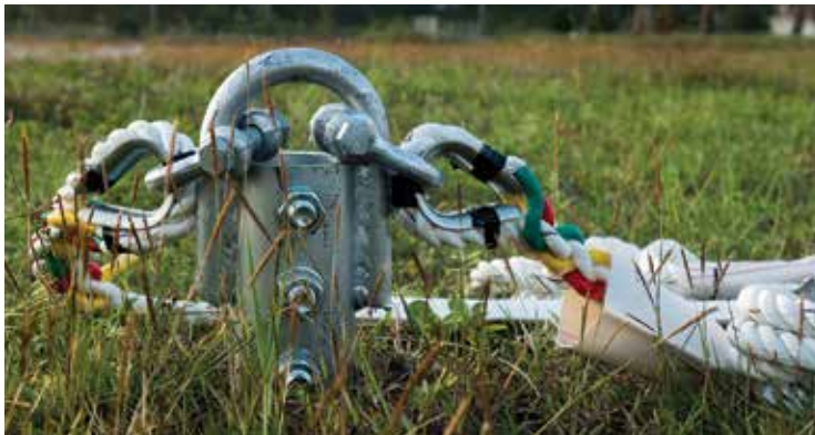
FIGURE 7.11 Land-based anchoring on the banks
