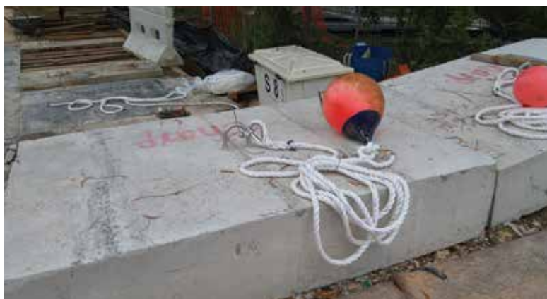
FIGURE 4.7 Concrete sinkers (left), and helical anchors (right)
