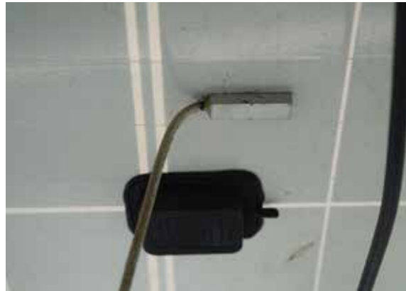
FIGURE 9.4 Examples of module temperature probes
