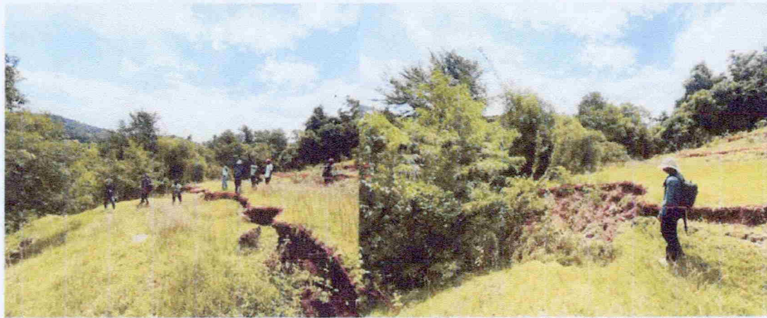
Figure 3 Terraces on the hillsides with vertical displacement of more than 0.5 meter. GPS Coordinates: 17° 17' 16.7"N 120° 32' 55.0"E
