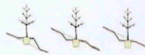
Figure 14. Planting on a slope. Too low: When planting on a slope, adjust the grade to plant "down-the-hill." Right: When planted "up-the-hill," roots on the uphill side will be too deep, slowing root establishment and growth.
